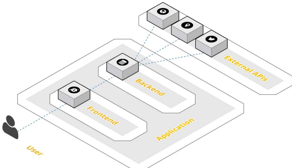
Figure 14 – Application architecture generated with CloudCraft
